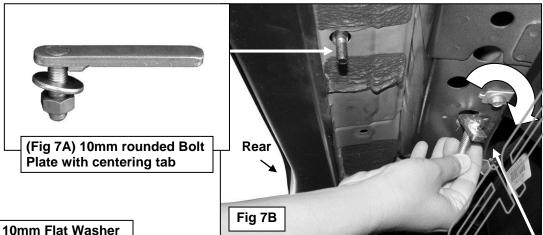
10mm Flat Washer 10mm Lock Washer 10mm Hex Nut
