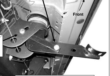
(Fig 8) 25-3500 Model Center Support Bracket Installation Pictured.
