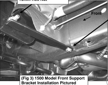
10mm Nut Plate 10mm x 30mm Hex Bolt 10mm Lock Washer 10mm Flat Washer
