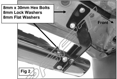
There are four sets of threaded holes in the side panel. Starting from the front of the vehicle, use the first, second, and fourth sets of holes.
