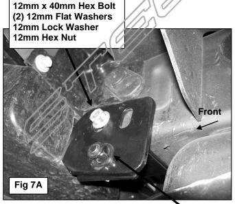
12mm x 40mm Hex Bolt (2) 12mm Flat Washers 12mm Lock Washer 12mm Hex Nut
