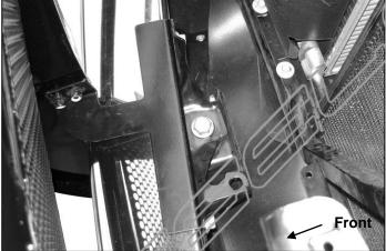
(Fig 10) Passenger side Top Bracket installation pictured from above
