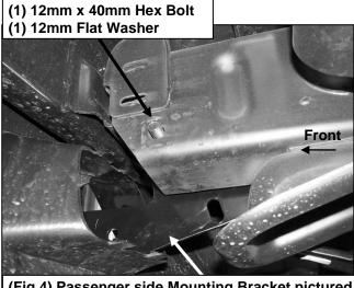
(Fig 4) Passenger side Mounting Bracket pictured
