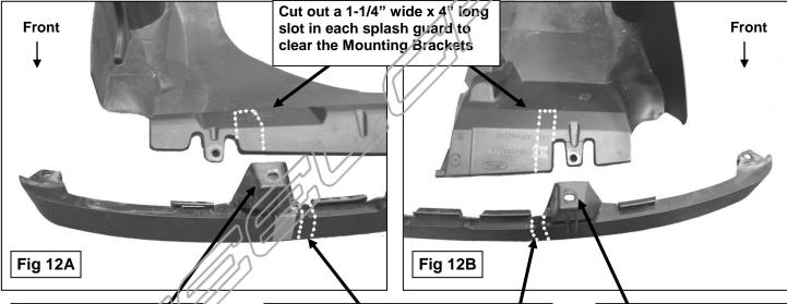
Replace factory hardware for this mounting location with the included. 6mm x 30mm Phillips Screw 6mm Lock Washer 6mm Flat Washer
