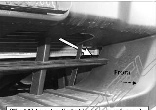
(Fig 1A) Locate clip behind bumper (arrow), at each end of bumper opening
