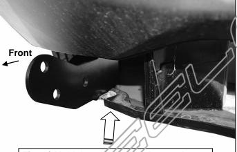
Fig 14) Hold the splash guard up to the bottom of Frame Brackets. Trace location of Brackets onto back of the plastic cover
