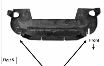
Trace location of Brackets onto back of the plastic cover (dashed line). Cut as required to clear brackets. Do not cut off mounting tabs and clips
