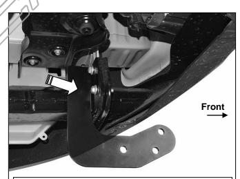
(Fig 6B) Use 12mm x 32mm Large Flat Washer for a spacer on lower mounting bolt only between Mounting Bracket and bumper bracket (Driver side Bracket installation pictured)
