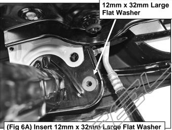
between Mounting Bracket and bumper bracket
