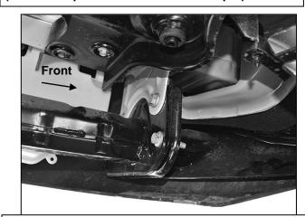
(Fig 3) Locate bumper bracket (driver side pictured)
