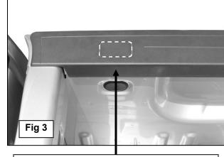
Follow the factory guide lines to cut out the cover over the front stake pocket. The guide lines in the cover may not represent the actual size of the stake pocket. Be very careful cutting through the plastic cover to avoid damage to the top of the bed.
