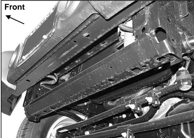
(Fig 1) Remove plastic splash guard from bumper
