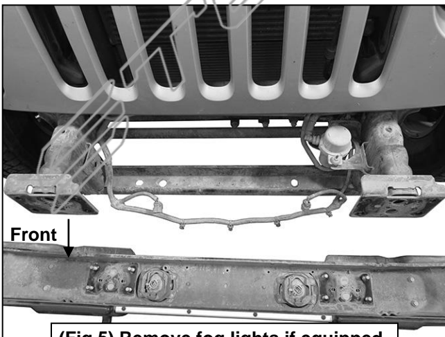
(Fig 5) Remove fog lights if equipped
