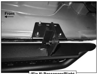
(Fig 8) Passenger/Right Rear Sidebar installed
