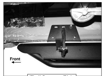
(Fig 6) Passenger/Right Front Sidebar installed
