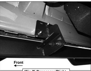
(Fig 7) Passenger/Right Center Sidebar installed
