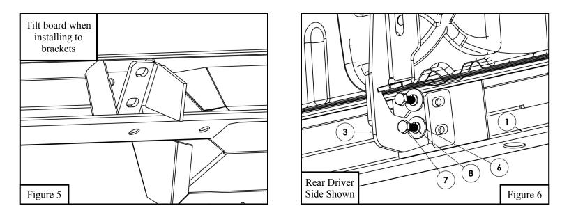
NOTE: For installation on diesel equipped vehicles. Follow the instructions on the following page for the diesel exhaust fluid (DEF) tank removal. This is located adjacent to the passenger side front rocker panel. This is necessary for the installation of the front mounting brackets for the passenger side.
