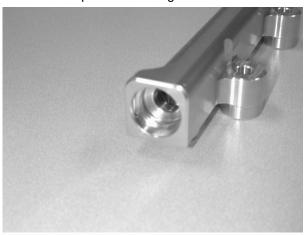
**b)** Make sure both ends of the fuel rail are clean and free of debris and burrs.
