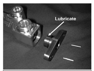
f) Lightly lubricate the tip of the end adapter and the o-rings in the end of the fuel rail. Clean engine oil works well.
