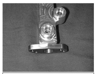
**g)** Insert and tighten two 1-2062 screws into the dowel pin holes. Repeat steps b-g for the other side of the fuel rail.
