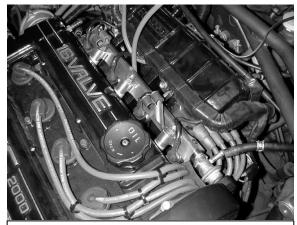
**e)** Install and tighten the three fuel rail mounting bolts. Make sure to reinstall the two throttle cable brackets on the outer fuel rail bolts.
