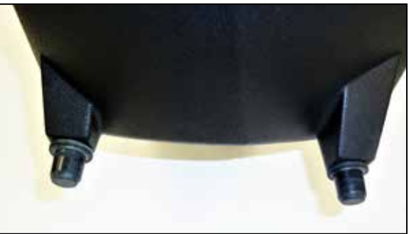
15. Remove the two-air box mounting grommets from the factory air filter housing and install them onto the AIRAID air filter housing as shown.
