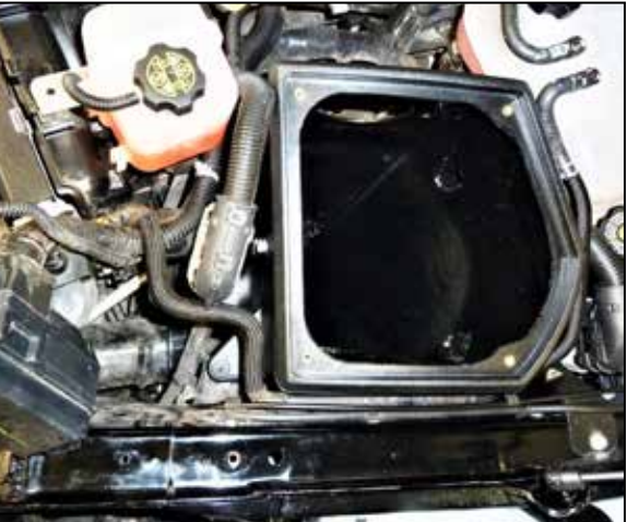
16. Install the AIRAID air filter housing into the vehicle so the mounting grommets insert into the factory mounting holes and then secure with the factory mounting nut.
