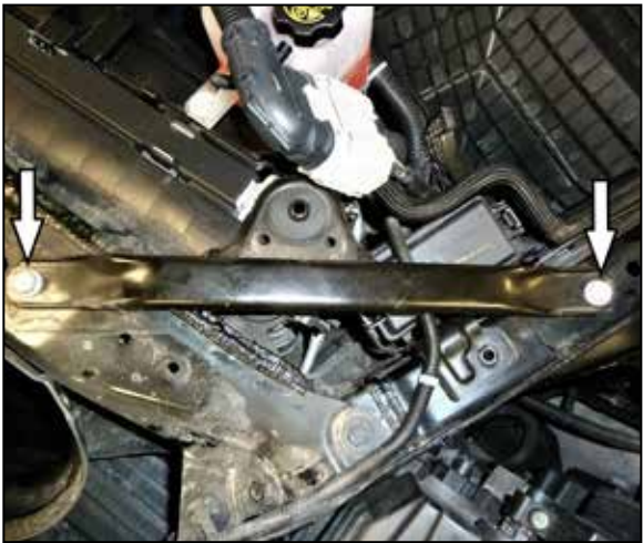
10. Remove the two bolts that secure the strut brace and then remove the strut brace from the vehicle.
