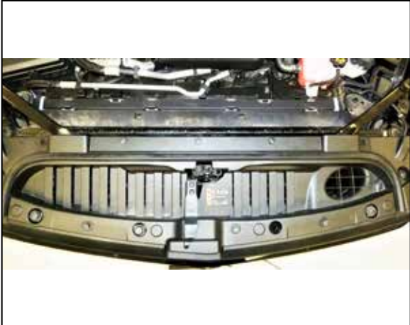
19. Reinstall the valence and secure with the factory retaining clips. Reinstall the hood release arm to the hood latch and secure with the factory bolts.
