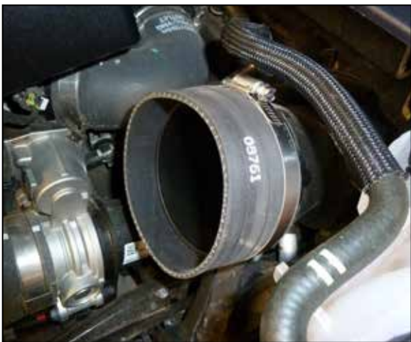
20. Install the provided coupler onto the turbo inlet and secure with the provided hose clamp.
