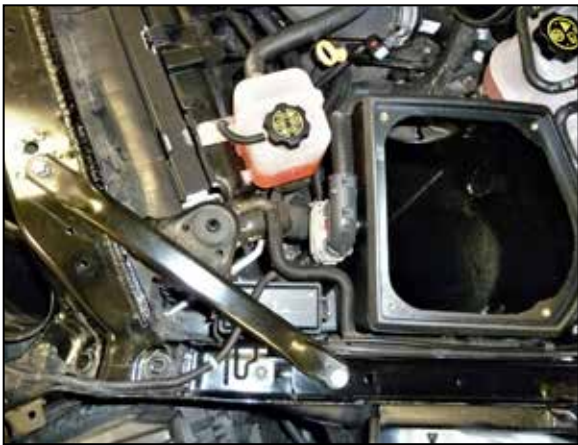
18. Reinstall the strut brace using the factory hardware. Resecure the relay box and expansion tank with the factory hardware.
