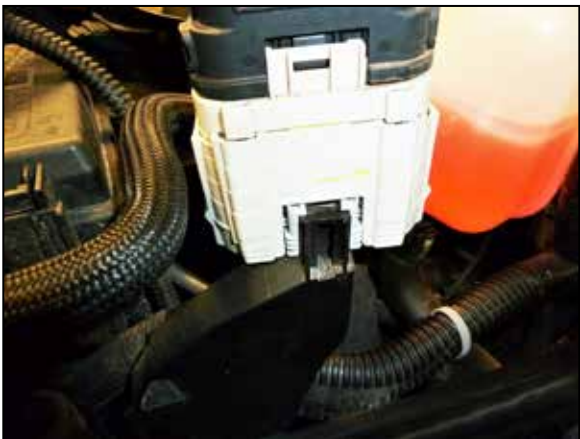
8. Release the locking tab and then disconnect the bulk electrical connection from the air filter housing.
