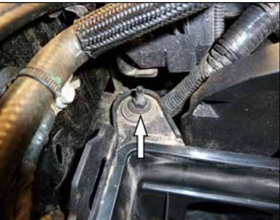
13. Remove the nut that secures the lower air filter housing and then remove the lower air filter housing from the vehicle.
