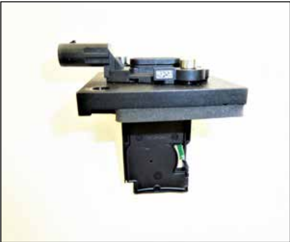
21. Install the provided gasket onto the mass air adapter. Remove the mass air sensor from the factory air filter housing and install it into the adapter and secure with the provided hardware.
