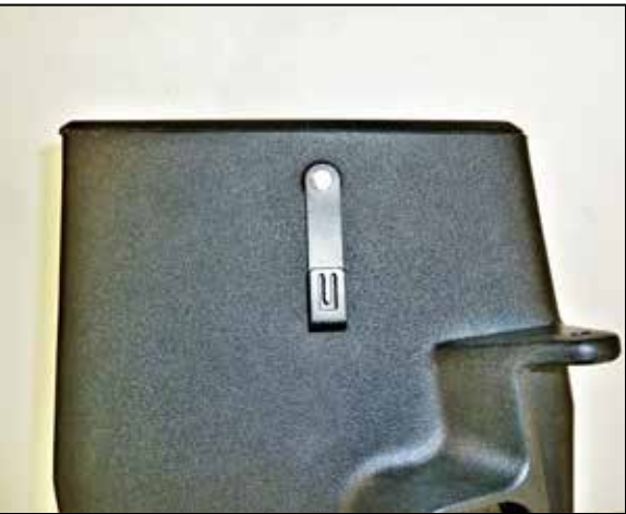
14. Install the wiring harness bracket onto the AIRAID air filter housing using the provided hardware.
