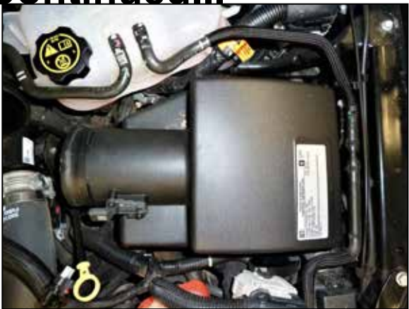
7. Loosen the three screws that secure the air filter lid onto the air filter base. Remove the lid and hose assemble and factory air filter from the vehicle.
