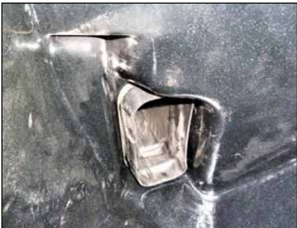
17. Engage the fresh air duct into the AIRAID air filter housing and then secure it with the factory retaining clip.
