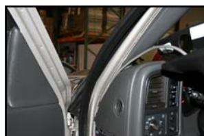
Run wires behind dashboard
