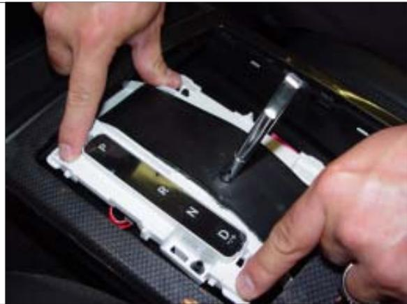
**STEP 9.** Remove the black plastic slider cover from the shift stick by simply pulling upwards and lightly bend the edges (front and back) downward.
