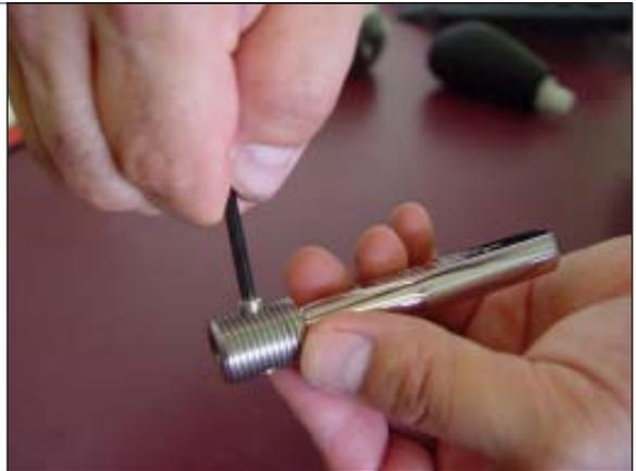
**STEP 15.** Slide the Hurst stick onto the original stock stick to where the top of the Hurst stick is flush with the original shifter stick and the threaded hole is towards the front of the vehicle.
