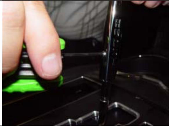
**STEP 17.** Attach the Hurst nut onto the threads of the Hurst stick. Screw it all the way down towards the bottom of the threads.
