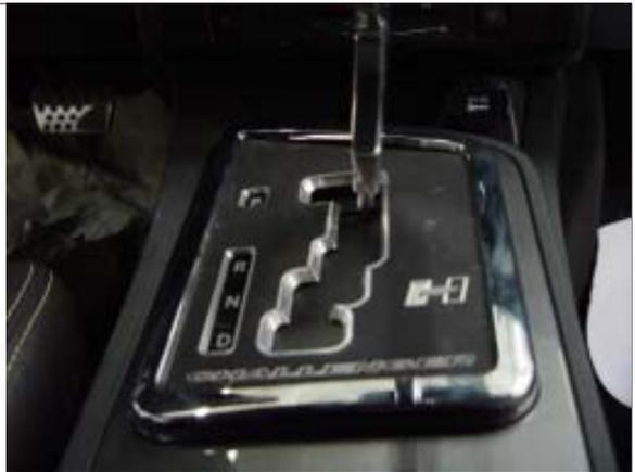
**NOTE:** You may notice a small hole in the HURST "H" This hole was intentionally added in order to access the parking lock switch. Use a straightened paperclip or bobby pin to access this hole. Avoid the use of sharp objects such as a needle or a pick. This switch should only be used when the vehicle needs to be taken out of park and when pressing on the brake pedal does not work. The brake pedal should always be used to take the vehicle out of park for all other instances.
