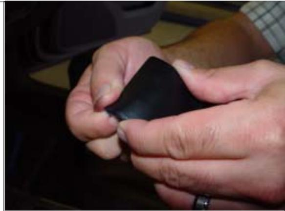
**STEP 10.** Tightly roll the black plastic slider cover (teeth inward) to put a permanent "curve set" into the plastic. Wipe away any grease that may have transferred to the top of the cover.
