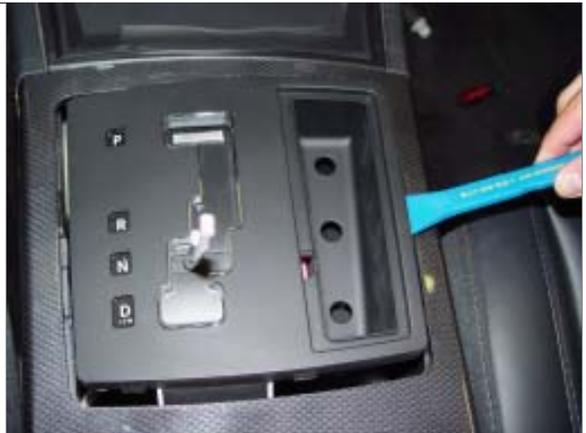
**STEP 6.** Gently pry the driver's side black attachment tabs (front and back) free from the white shifter housing.
