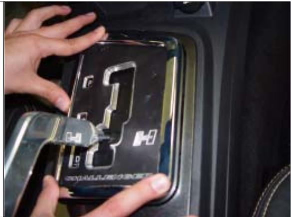
**STEP 21.** With the key in the ignition (vehicle "OFF") and foot firmly depressing the brake pedal. Cycle the shifter through all position to ensure smooth and accurate movement. If binding or rough movement occurs, review and ensure that STEP 9 & 10 has been completed or needs to be revisited.
