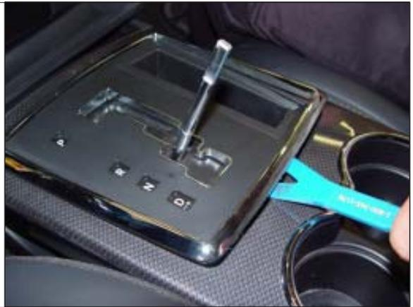
**STEP 5.** Carefully separate the black plastic shifter face plate from the shifter by gently prying up from the passenger side.
