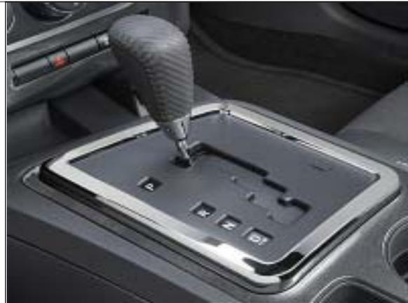
**STEP 2.** Carefully pry the chrome knob collar down away from the knob and push it down off of the knob.
