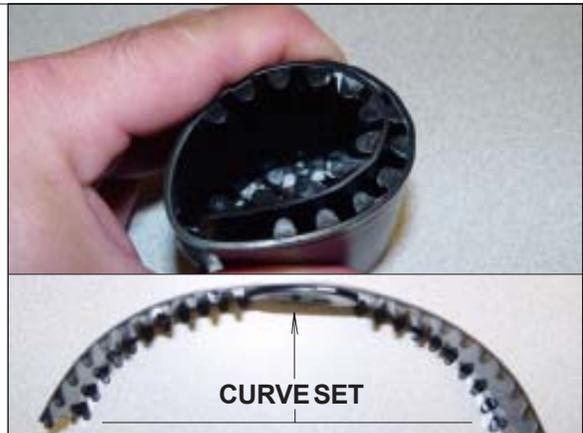
**STEP 11.** Replace the black plastic slider cover remembering where the nub was originally located.
