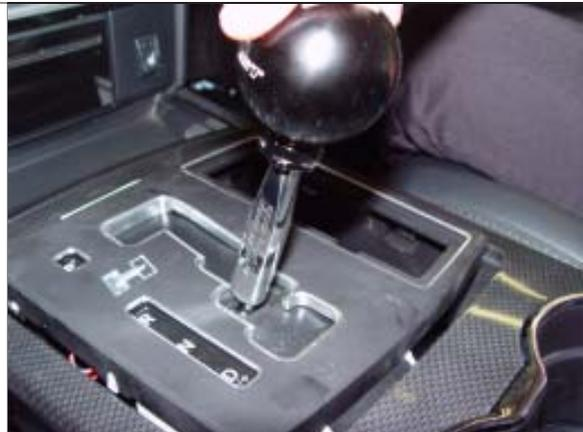
**STEP 19.** Tighten or "jam" the Hurst nut up against the Hurst knob while holding the correct Hurst logo position.
