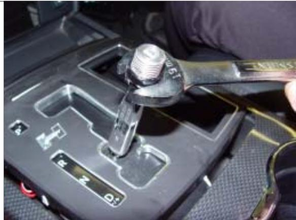
**STEP 18.** Screw on the Hurst knob all the way down until it contacts the Hurst nut. Then unscrew the knob until the Hurst logo aligns correctly.
