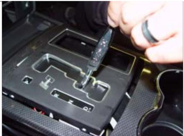
**STEP 16.** Starting with the top two (2) screws, tighten all three (3) of the set screws to ensure the Hurst stick stays secure onto the original shift stick.
