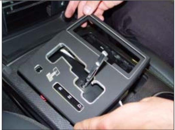
**STEP 13.** With the tabs in place from STEP 11, firmly push down on the passenger side of the Hurst plate to snap into place.
