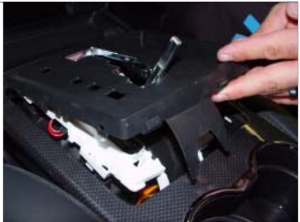
**STEP 8.** Ensure that the white shifter housing has not unsnapped free from the shifter by pressing down and snapping back into place on the shifter if it has become loose.
