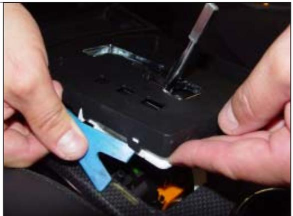
**STEP 7.** Remove plastic shifter plate by lifting the rear out from the center console and then sliding the plate back to free and remove the plate.
