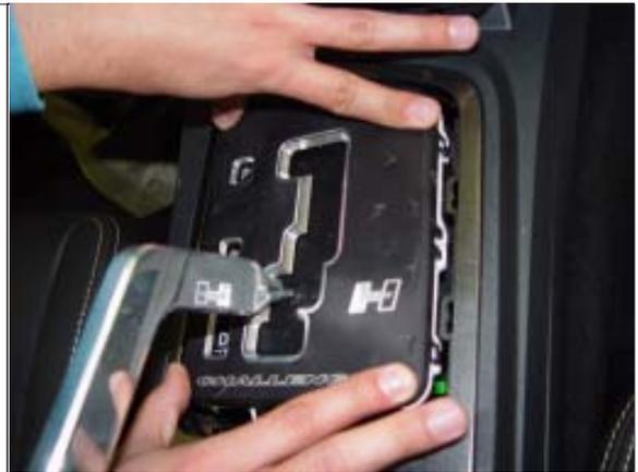
**STEP 14.** Start the three (3) set screws into the three (3) threaded holes on the stick (two on the threads and one on the front).
