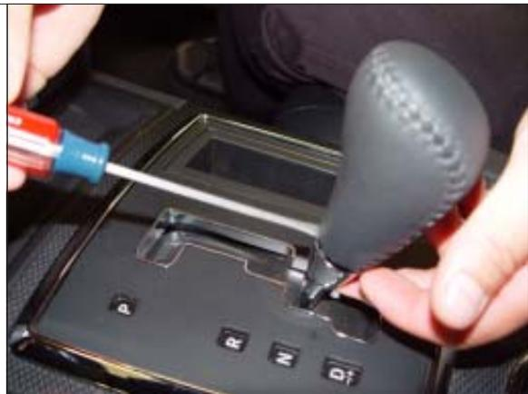
**STEP 3.** Pull up sharply on the knob to remove it and also remove the collar.
