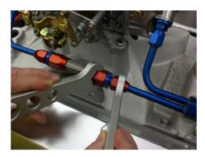
6. Using a wrench to secure the flex connection assembly from turning (use **CAUTION** here so that the flex connection assembly does not slide) tighten the tube nut. Follow the same procedure for the rear feed line.
