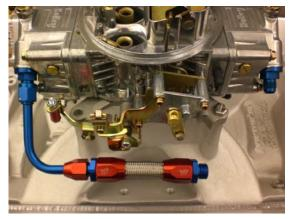
Slide the flex connection assembly over rear feed line and snug up on tube nut. <u>DO NOT</u> tighten tube
