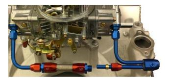
Install front feed line onto front float bowl. Slide one compression nut and one compression sleeve Onto the feed line.
