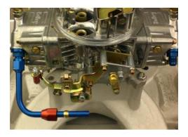
2. Install the rear feed line into the rear float bowl. Slide one compression nut and one compression sleeve onto the feed line.
