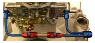
5. Slide the flex connection assembly over front feed line and snug up on tube nut. **DO NOT** tighten tube nut. Center flex connection assembly between front and rear feed lines.
