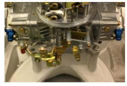
1. Install carburetor adapter fittings onto float bowls.
