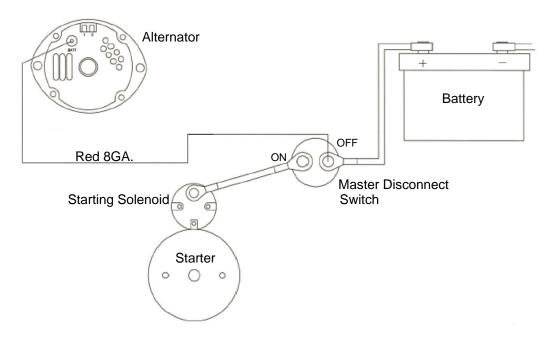
**CHECK FOR PROPER SHUTDOWN OPERATION BEFORE DRIVING VEHICLE:** Any time the master disconnect switch is in the 'OFF' position the car should NOT run.
