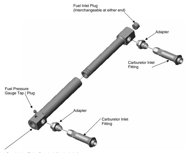
Fuel Supply Inlet Fitting Required (Not Included)
