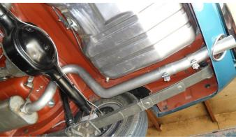
7. If you are using the s-bend extensions, there is a bolt on the shackle of the spring that you may either need to trim shorter or flip the head of the bolt around to allow for proper clearance of the s-bend extension pipes. See before and after trimmed bolt in the pictures below. You may also flip the bolt around and have the head of the bolt towards the s-bend extension pipe. Trim or flip the bolt as desired if necessary.
