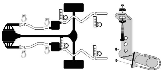
Hanger consists of a metal strap, grommets, hardware and clamp (see illustration).
