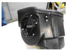
**Step 8.** Locate #3 "L" bracket. Install "L" bracket to JEGS air box. Using the supplied 10-32 SS machine screws, fasten the bracket to the front side of the JEGS air box. \*Note: Install the head of the machine screws from the outside of the air box.
