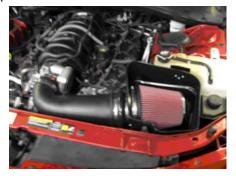
**Step 13.** Locate #2 Hood Seal. Install the air box hood seal. Using the supplied hood seal, install the seal around the top of the JEGS air box assembly.
