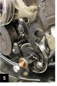
5. Verify the fit of your belts with the bracket positions; tighten all bolts/nuts and adjust the belt tension as normal.
