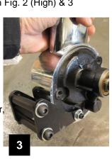
4. Loosely attach the adjusting arm bracket to the front of the pump and the engine. For "long" water pump applications, the dogleg in the bracket goes towards the engine; for "short" water pump applications, the dogleg points away from the engine. A 1/8" washer may need to be used between the spacer on short pumps as well. (Fig. 5)
