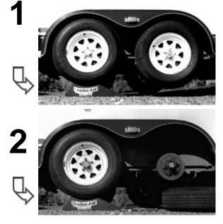
Slightly loosen lug nuts on bad tire. Drive your good tire onto Trailer-Aid. This will lift your flat tire off the ground.
