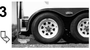
Drive off Trailer-Aid®, tighten lug nuts securely, and you're on the way.
