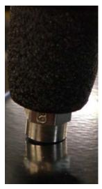
9. Unscrew the Mandrel from the Rivet Nut by loosening the Thumb Screw.
