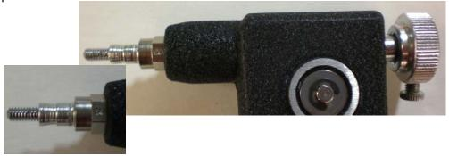
8. Press the Rivet Nut into the desired hole and actuate the gun handle.
