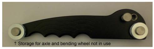
To bend tubing, insert into desired axle and bending wheel. Firmly hold tubing against axle while bending around wheel to desired position. Be sure that tube does not slide or move. Also, be sure to us appropriate wheel for the size tubing you are bending.
