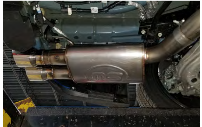
Detail 12a: Left muffler assembly installed
