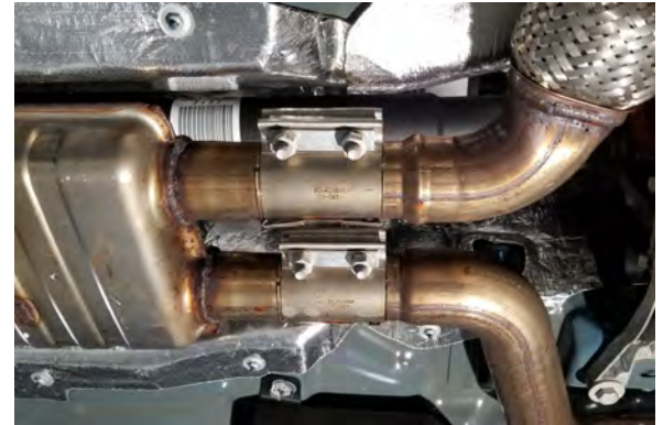
Detail 3: Clamps at catback connection
