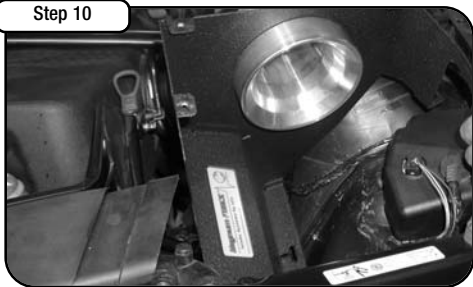
Using 10mm socket replace headlight controller using original bolts and provided spacer on lower tab. Place heat shield into engine compartment, placing slot over the bolt that originally secured the rubber mount.
