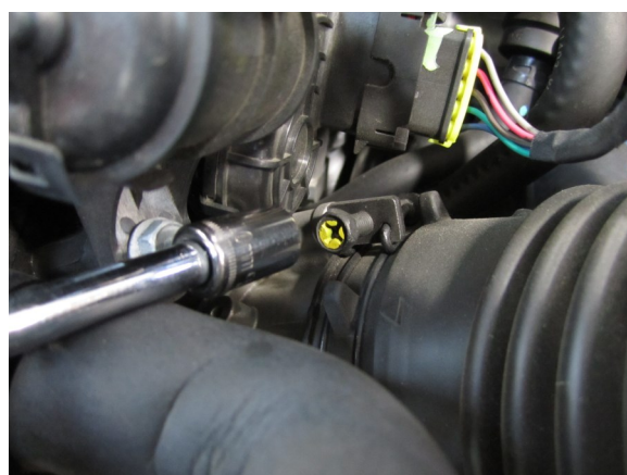
D. Loosen the hose clamp at the throttle body.
