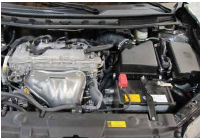
a. Stock airbox system installed.
