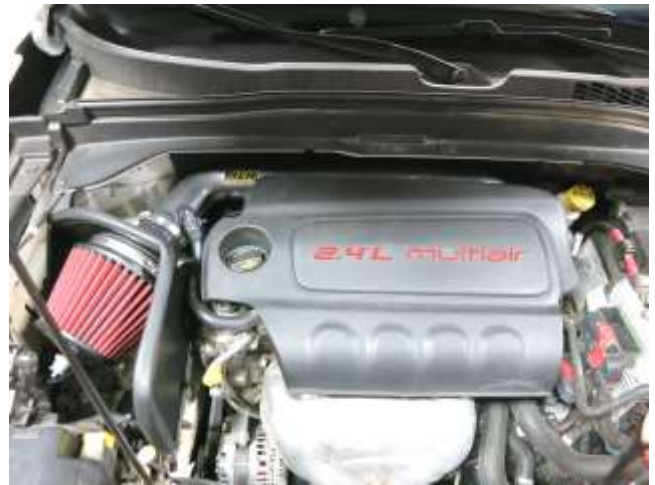
p. Finished installation of AEM Intake System.
