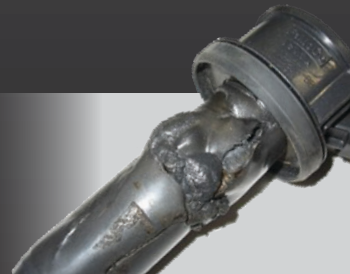
Figure 1: Failed ignition coil in a Ford application.
