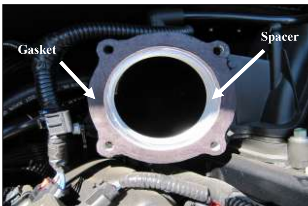
5. Insert the Airaid spacer into the intake manifold. The gasket will go between the spacer and the throttle body. *Note: Airaid spacer must be installed with bore protruding into intake manifold away from throttle body. Incorrect installation will hinder performance. Reference picture below for spacer orientation.
