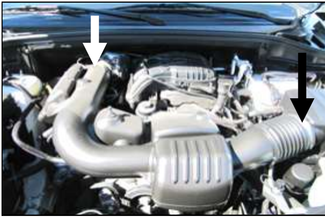
3. Loosen the clamps on both ends of the intake tube, and remove from the engine compartment.
