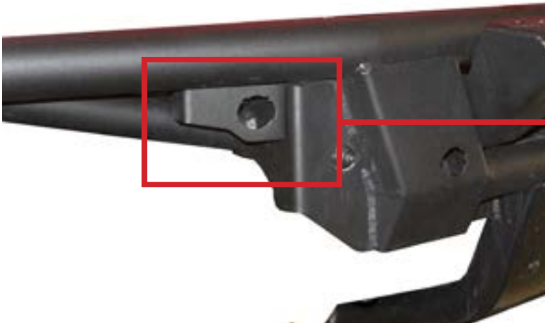
Fig V Have The Lock Nut Side Faced Out By Sensor
