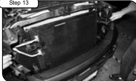
Re-install intercooler to radiator support. (step 5) Re-attach a/c condensor and cover and tighten. (step 2)
