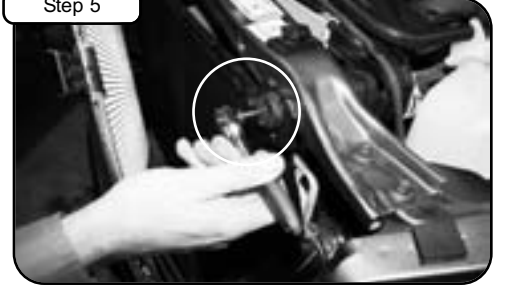
Loosen the two 10mm screws holding in intercooler on radiator support.
