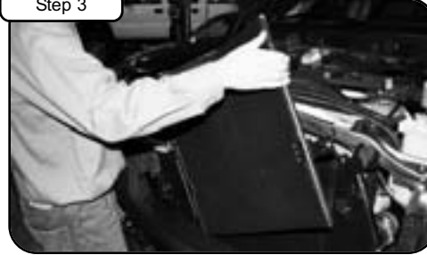
Pull up condensor only on the driver side.
