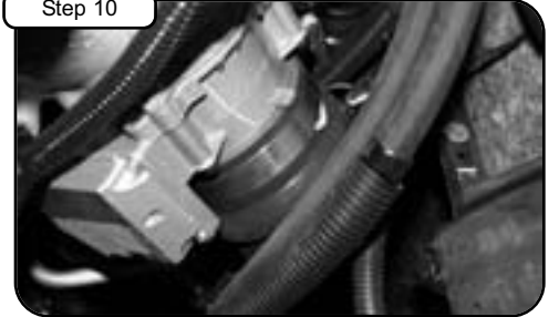
Install 3-1/2" hump coupler to manifold with clamps provided.
