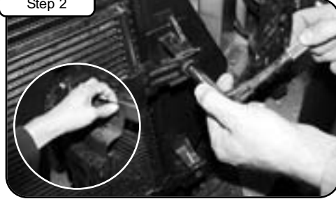
Loosen the four bolts holding in a/c condensor. Pull back passenger side condensor cover.
