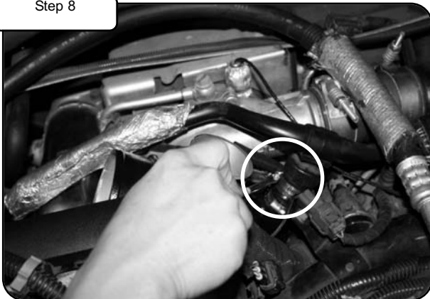
Re-attach CCV hose coupling on aFe turbo inlet tube using supplied mini hose clamp. Tighten with flat tip screwdriver or 1/4" socket driver. Re-attach CCV hose end on passenger side of truck.
