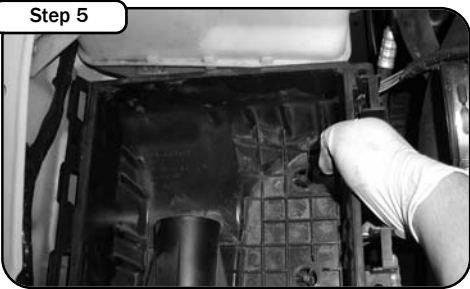
Lift up and remove bottom half of air box.
