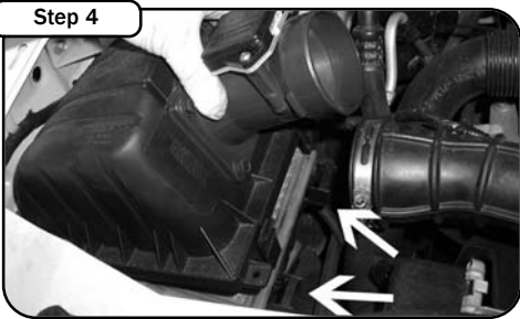
Depress the two mounting tabs located on the side of the airbox. Lift the top half of the airbox out and remove..
