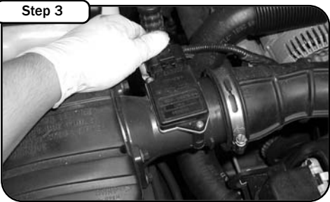
Disconnect negative post from battery terminal. Loosen the hose clamp on the intake duct. Disconnect the MAF sensor by pushing down on the clip and pulling out.
