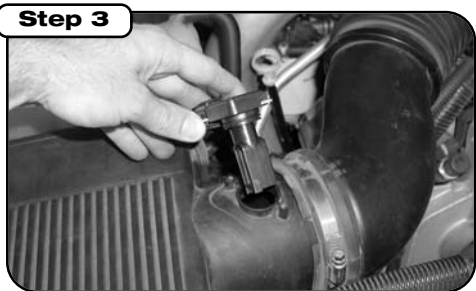
Remove two screws that hold mass air flow sensor to stock airbox using supplied torx bit and remove sensor from airbox.
