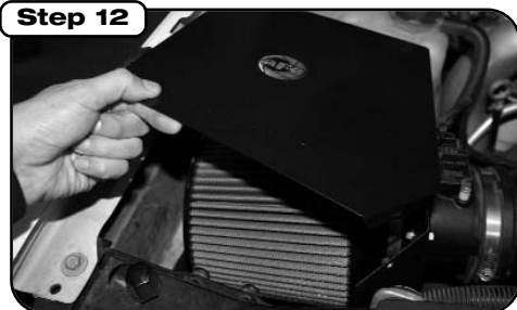
Place cover on top of housing and fasten securely using 3 supplied 1/4-20x3/4 bolts and washers. For stage I kits, make sure all clamps are tight and all components are secure. Check and retighten connections and filter after a few hours of operation. (End of stage I installation instructions.)
