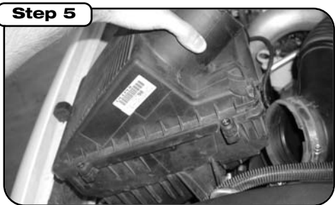
Remove the complete stock airbox from the rubber mounts. Pull up and slide sideways toward radiator.
