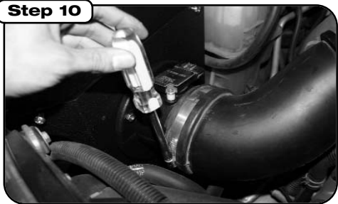
Reconnect stock intake tube to Housing. Fasten securely. Also reconnect MAF sensor harness.
