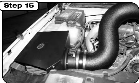
Place the included CARB EO Sticker on or near the intake system on a smooth, clean surface. E.O. identification label is required in passing the Smog Check Inspection. Complete Stage 2 kit installed. Make sure all clamps are tight and all components are secure. Check and retighten connections and filter after a few hours of operation.
