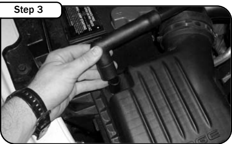
Remove crank case breather line from airbox and oil fill chamber.
