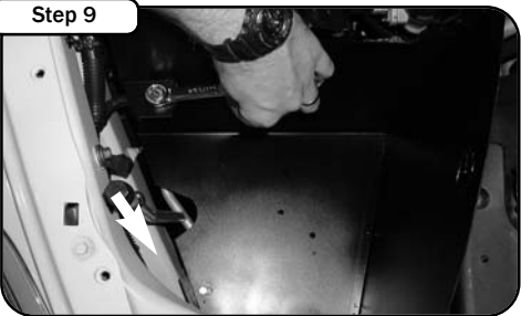
Place intake housing into vehicle and fasten down securely reusing core support screw from step 7 and use M6 x 1 x 12 for the bottom screw.
