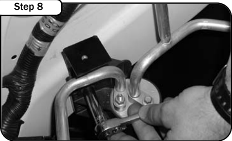
Loosen screw but do not remove completely. Slide bracket that was supplied in the kit into place and retighten screw. This new bracket is placed in between the accumulator bracket and side fender well.
