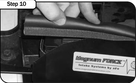
Install trim seal onto intake housing.
