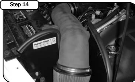
Complete kit installed. When servicing filter, intake tube and attached filter must be removed as one assembly. Securely tighten all connections and re-check as necessary
