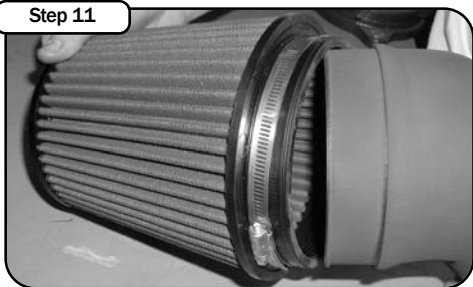
Install filter onto end of intake tube and fasten securely. Also place coupler onto end of resonator and fasten securely.
