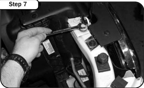
Remove 13mm screw from radiator core support. This will be reused once heat shield is installed.
