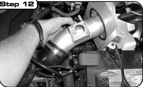
Install provided coupling to the throttle body, with the shorter of the two ends connected to the throttle body. Place, but do not tighten clamps on both ends of the coupling and install provided aluminum intake tube into the coupling and through the heat shield opening. (Note: 1zz motor uses part # 05-00135 with ID of 2.75", 2zz motor uses part # 05-00136 with ID of 3" to 2.75")
