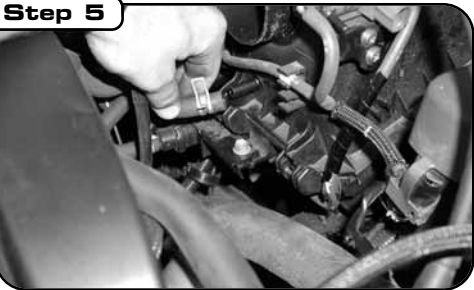
With intake tube now removed, there is a 3/8" vacuum line connected to lower portion of airbox and leading the lower VSV. Disconnect this line from the lower airbox.
