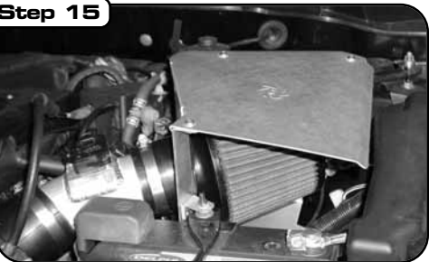
Install heat shield lid. Securely tighten all connections and re-check as necessary.
