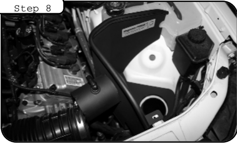
Lower housing into engine bay. Make sure the tab on the back of the housing slides into the slot on the side of the radiator reservoir. Be sure to clear rubber hose near bottom of housing.
