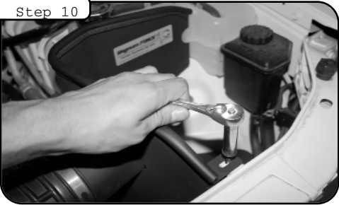
Align the mounting holes on the housing. Secure the assembly with the factory hardware.
