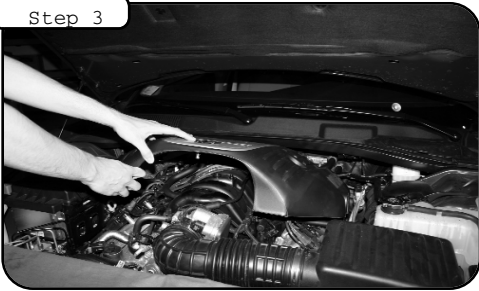
Disconnect negative terminal from battery. Lift off Hemi engine cover. Disconnect the breather hose on the side of the valve cover.
