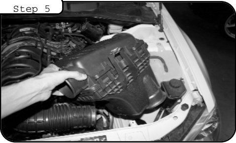
Remove the factory air box assembly.
