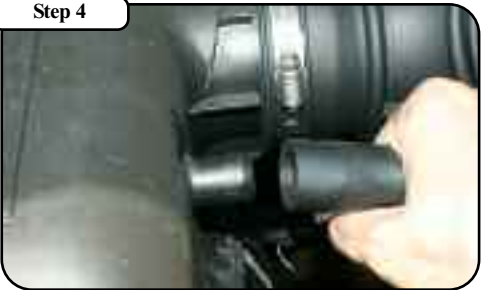
Unplug the crank case breather tube.
