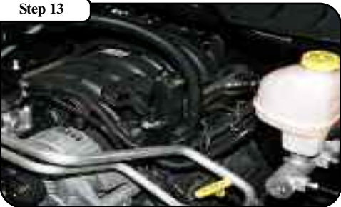
Replace old crank case breather line with the hose provided and run in direction of the OEM line and put the engine cover back on. Remember that the engine cover has a slot where this line will come out from.
