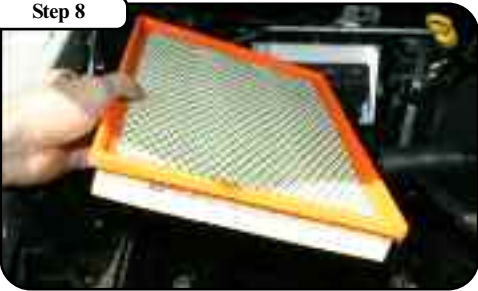
Remove the stock air filter.
