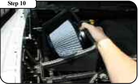
Place aFe housing and filter into the stock OEM Airbox and clip all four clips to secure housing.
