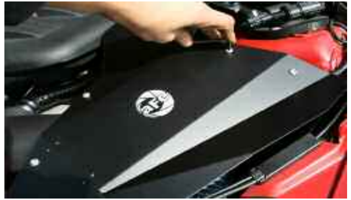
29- Secure cover with supplied M6 button head screws and tighten with 4mm allen wrench.
