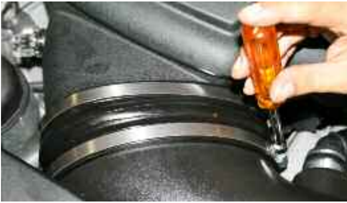
25- Tighten clamps on supplied coupler using a 5/16" nut driver to secure intake tube to intake manifold. Note: Do not over tighten.
