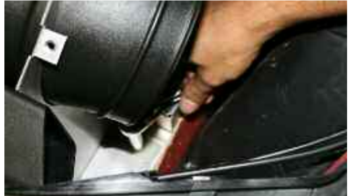
22- Tighten lower housing support nut with 10mm socket or wrench.
