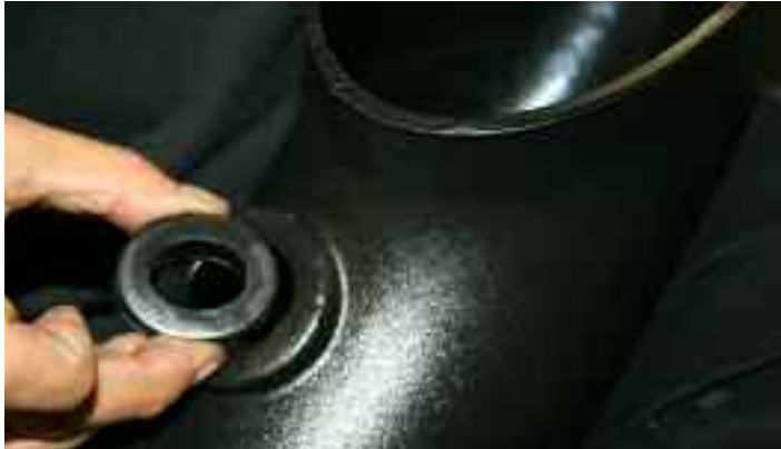
10- Install supplied grommet into aFe's intake tube.
