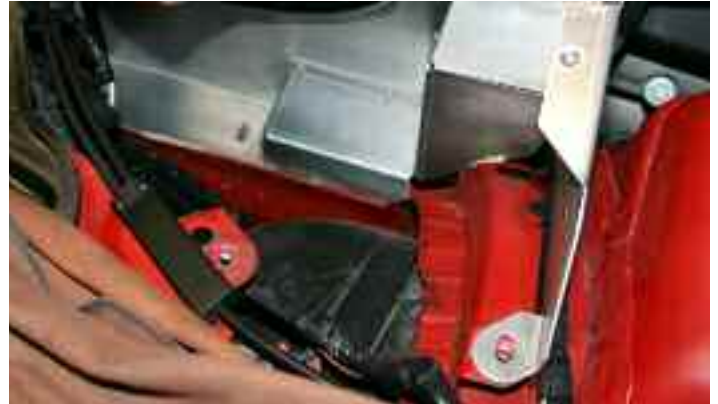
14- Carefully position housing into the vehicle and line up the mounting points. Do not tighten housing.
