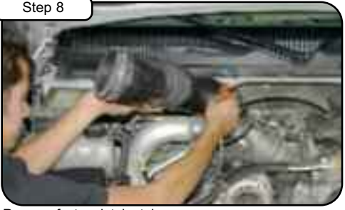
Remove factory intake tube.
