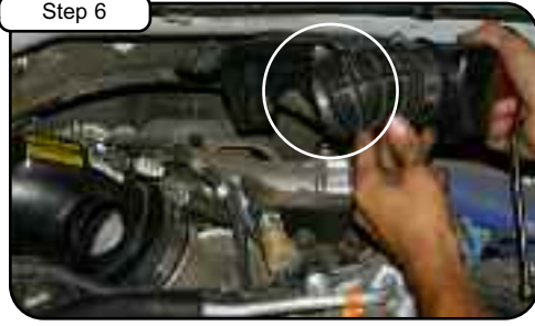
Cut clamp on resonator box connected to factory intake tube and pull back. Replace with mini # 040 clamp provided (see step 18). Do not tighten.
