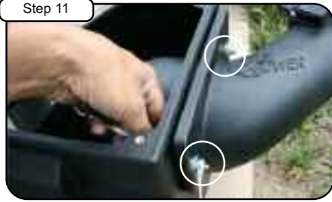
Attach tube to outside of housing using screws, nuts and fender washers provided and tighten using 7/16" socket or wrench.
