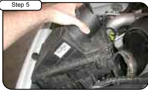
Lift and pull air box out of vehicle.
