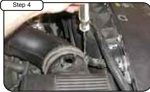
Loosen clamp on air box with 5/16" nut driver.
