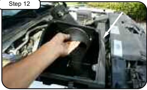
Install housing with tube into vehicle and position.
