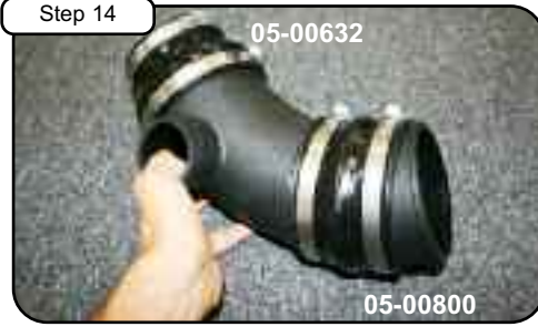
Attach reducer coupler (05-00632) to tube with clamps and hump coupler (05-00800) with clamps. Pull back hump coupler for easier installation. Do not tighten.
