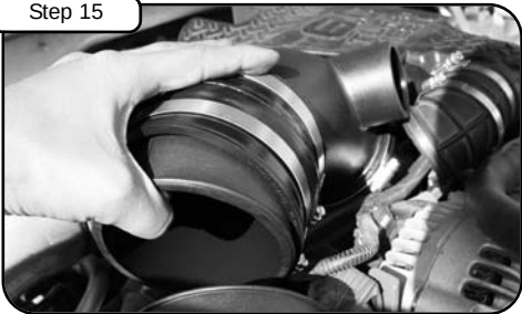
Install tube to turbo inlet flange and position. Make sure reducer coupler is on turbo flange. Do not tighten.
