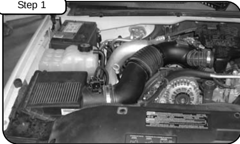
Complete Stock Intake. Disconnect battery before install.
