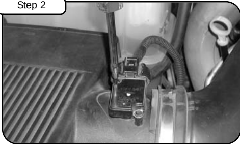
With T20 torx bit provided, loosen the two screws holding in MAF sensor.
