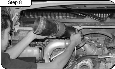
Remove factory intake tube.
