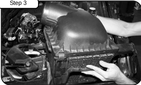
Disconnect air temp & MAF sensor. Loosen 10mm nut holding in front of air box using wrench or socket. Lift up and pull OE air box out of vehicle.
