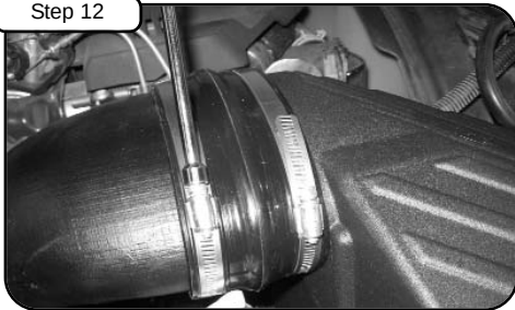
Tighten clamps at upper-cover with 5/16" nut driver.
