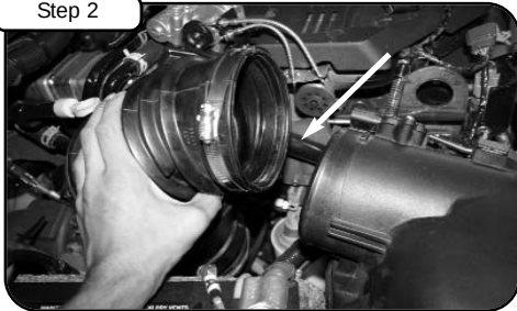
With 5/16" nut driver loosen clamps on OE tube at turbo/air box and remove. Loosen clamp at turbo and disconnect crank case line with pliers. Remove tube.
