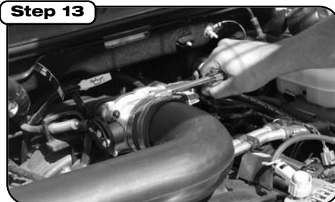
Slip coupler over throttle body and tighten clamps.
