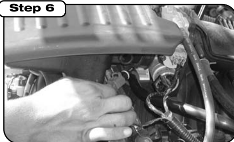
Remove temperature sensor from drivers side resonator box. Save for reuse. Note: Early 2002 V8-4.7L may not have temperature sensor in tube.
