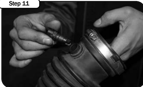
Remove the air temp. sensor from the OEM intake tube.
