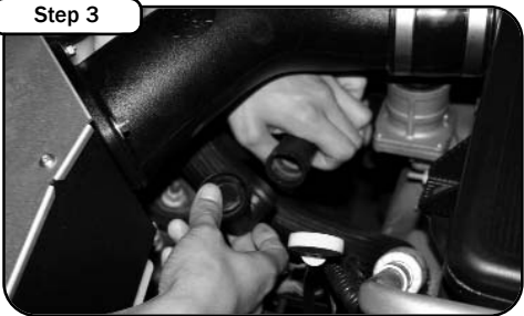
Remove the vent tube connector from the air injection hose.
