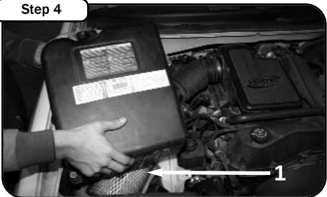
Remove the air box housing. (1) Remove the stock air filter.
