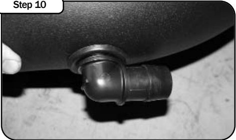
This is a sample photo of how the elbow should be inserted into the aFe intake tube.
