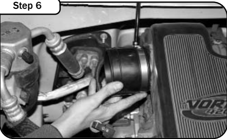
Slip the coupler over the intake manifold and secure with a clamp.
