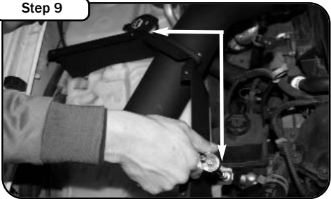
Fit the aFe housing over the intake tube. Using 2 screws, washers and lock washers secure the housing in the engine compartment.
