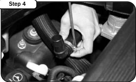
Using the #12 clamp and supplied vent elbow, secure onto the air injection hose.
