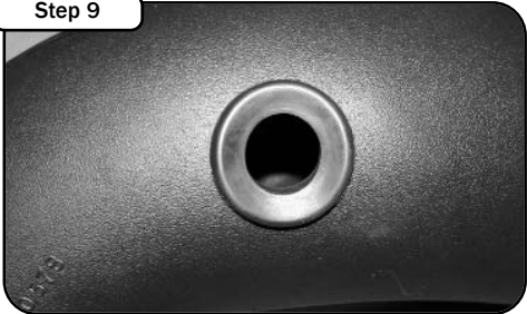
Insert the grommet so that its sits securely in the hole.
