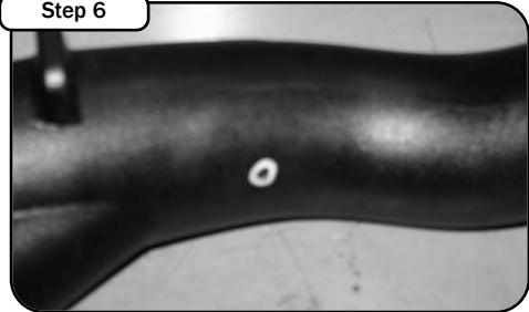
Now with the center marked, remove the aFe intake tube.
