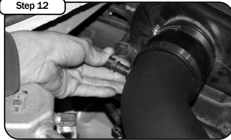
Insert the air temp. sensor into the aFe intake tube. Re-connect the air temp. sensor plug.
