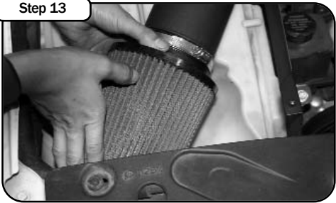
Install the new aFe air filter onto the intake tube and secure.
