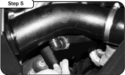
Position the elbow so it sits inline under the intake tube. Mark the center of the location.
