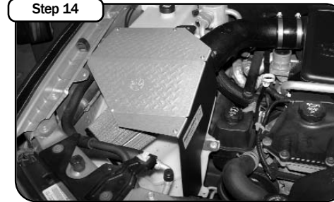
Position the housing cover and secure in position using 4 button head screws. Your installation is now complete. Make sure you tighten all clamps and check all electrical connections. Re-check periodically.
