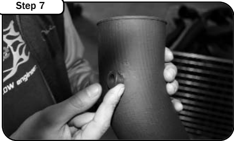
Insert the "air temp. sensor grommet" into the aFe air intake tube
