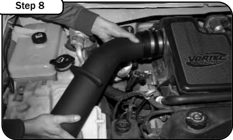
Insert the aFe air intake tube into the coupler on the intake manifold. Once in position secure the tube using a clamp.
