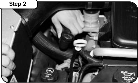
Using wire cutters remove the factory metal clamp from the air injection hose.
