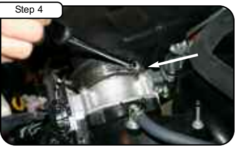
With 5/16" nut driver loosen both clamps on OE intake tube. Remove crankcase and vacuum line away from tube. Disconnect MAF sensor harness & remove.
