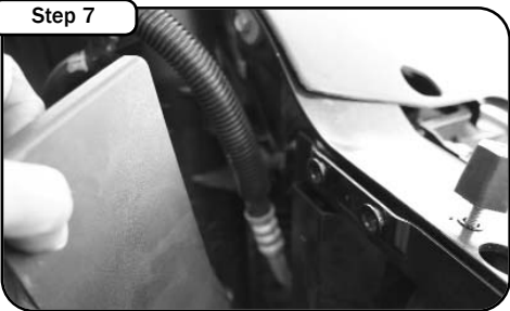
Remove plastic cover behind passenger head light.
