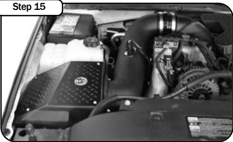
Place the included CARB EO Sticker on or near the intake system on a smooth, clean surface. E.O. identification label is required in passing the Smog Check Inspection. Your installation is now complete. Check all clamps and connections. Periodically check all clamps and hoses.
