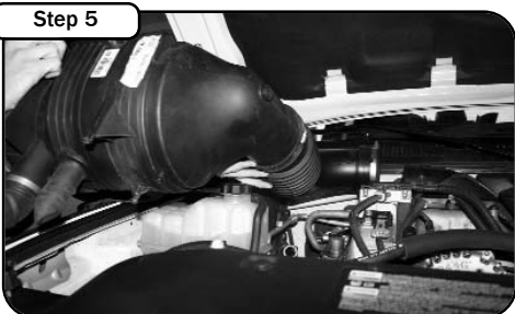
Carefully grab and pull out OE intake system from vehicle.
