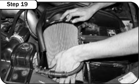
Install filter onto tube. Tighten clamp.
