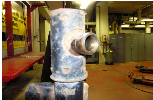
FIG 3, Strut Solenoid Removed
