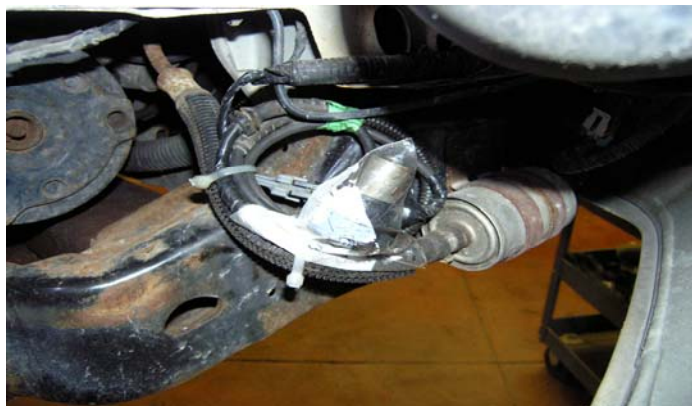
FIG 6, Solenoid Removal on Rear Shock
