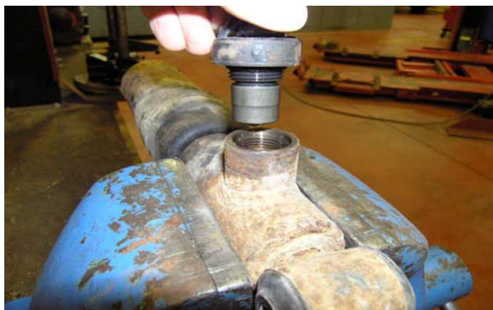
FIG 7, Rear Shock Solenoid Removed
