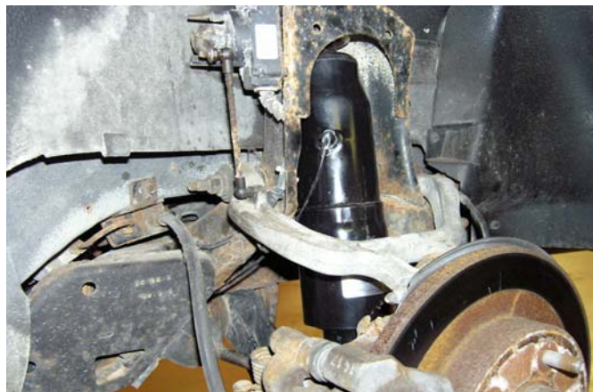
FIG 10, Rear Shock Installed Upper Portion Right Side
