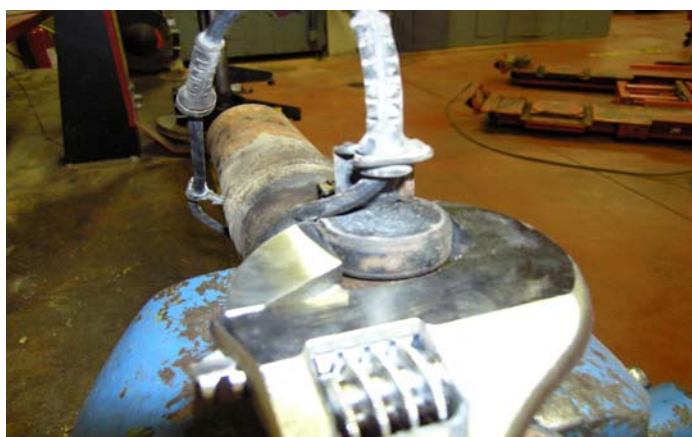
FIG 7, Rear Shock Solenoid Removed
