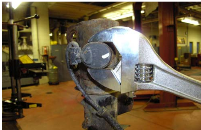
FIG 3, Strut Solenoid Removed
