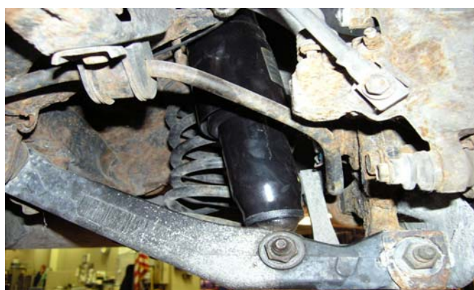
FIG 10, Rear Shock Installed Upper Portion Right Side
